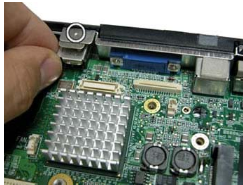
Fig. 31 Removing the AC socket holder
